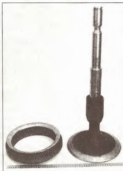
Figure 6. Seat and discharge valve of 258 mm diameter of the main engine of «Geroi Shipki» type ferry, surfaced with stellite (repair surfacing)
