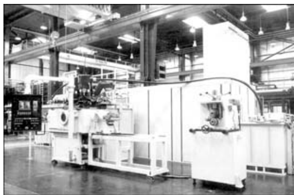
Figure 4. Batch-produced Steigerwald Strahltechnik unit of air-vacuum-air type for EBW of bimetal blanks
