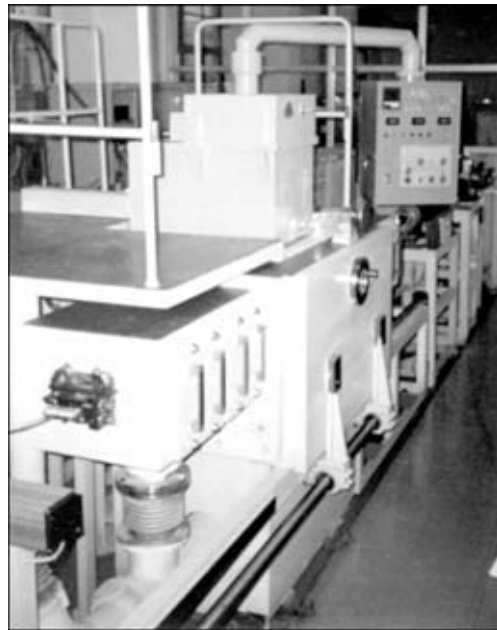
Figure 8. General view of the unit for EBW of a bimetal strip put into operation in Shanghai (China)
