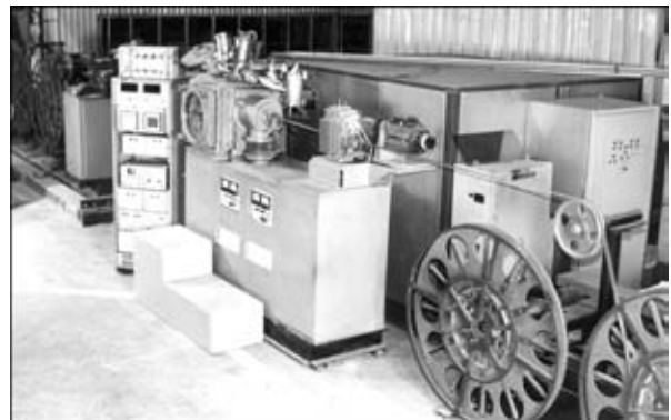
Figure 6. ELS-101 unit for welding of bi-, trimetal strip blank (developed by PWI)
