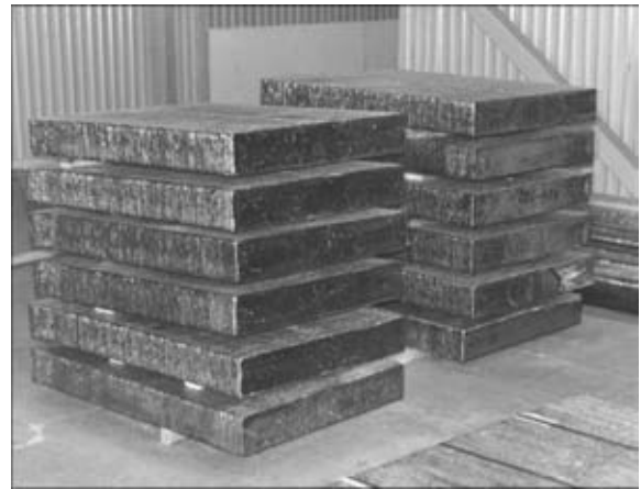
Figure 7. Slab ingots of VT1-00 alloy of 160 × 950 × 2000 mm size produced by EBMIC process
