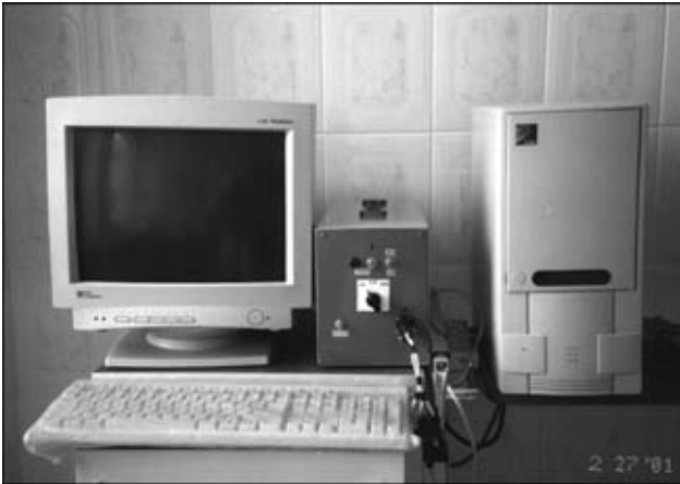
Welding complex for joining soft vital tissues
