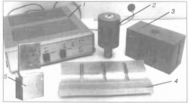
Figure 4. General view of an ultrasonic generator (1), piezoelectric converter (2), waveguides (3 - 5)
