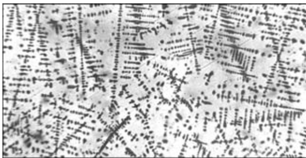
Figure 3. Microstructure of deposited bronze Br.AZh9-4 (x200)
