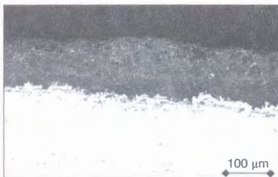
Figure 6. A layer on the inner surface of the cylinder, produced by simultaneous oxidising and abrasive treatment
