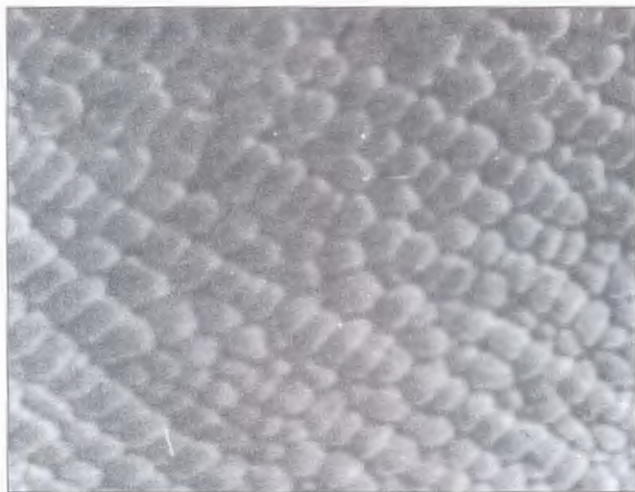
Figure 2. Microstructure of a section surface-melted by the electron beam in the zone of defect restoration ( \times 1740 )
