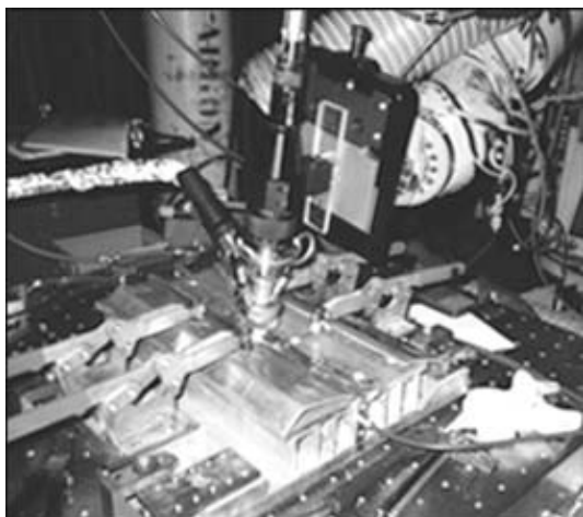
Figure 3. Integrated plasmatron with the laser focusing system connected to it
