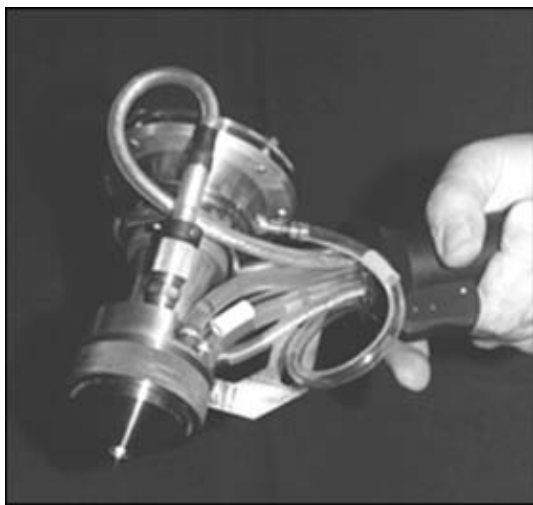
Figure 1. Integrated plasmatron for microplasma, laser and hybrid welding in automatic and manual modes
