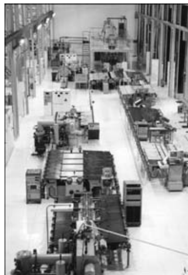
Figure 3. Automated line for fuel element sealing, based on the resistance welding unit
