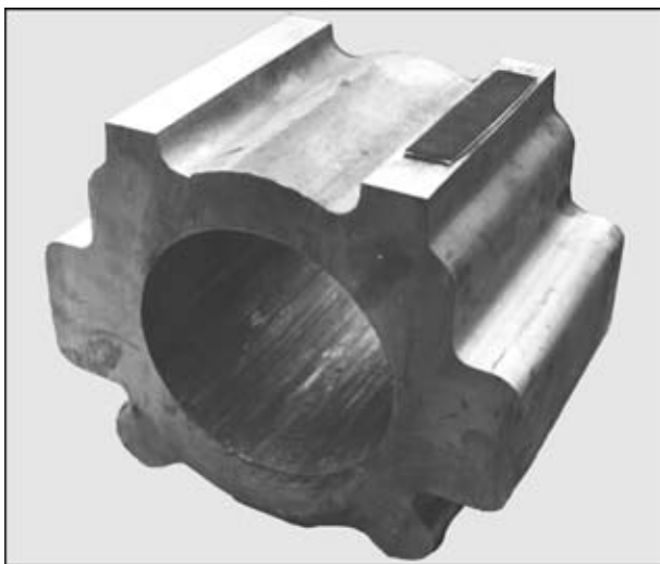
Axle box body with steel plate welded to it
