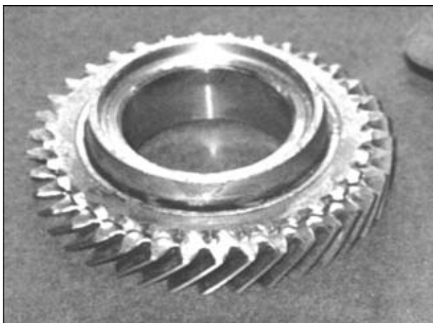
Figure 5. Appearance of the VAZ car gear ( D = 80 mm) welded using the TK-2.5 laser (welding speed — 2 m/min, focal distance — 150 mm, material — steel 18KhGT and 12Kh2N4A)
