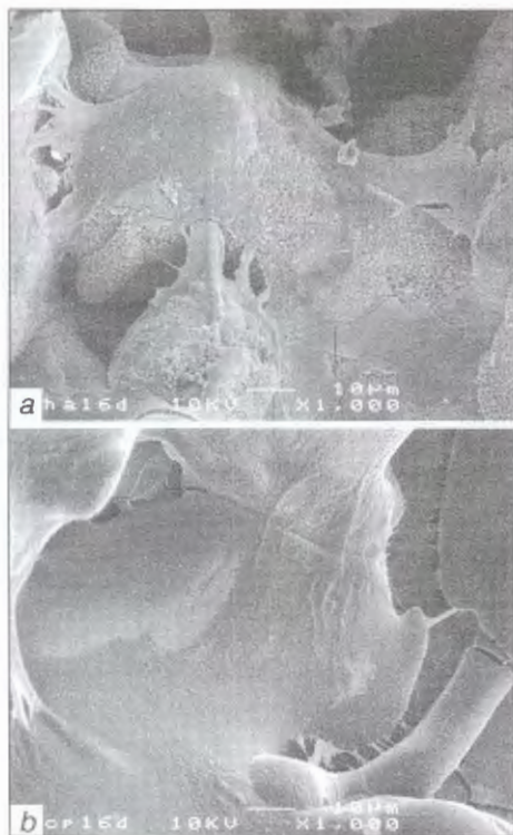
Figure 3. Appearance of the HAP (a) and TCP (b) bioceramic coatings with cell cultures
