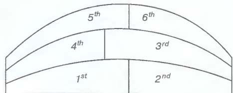
Figure 3. Schematic of assembly of a three-lobe block: 1 st –6 th — lobes
