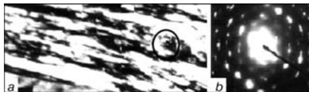
Figure 3. Fine structure of the nickel welding zone (a) resulting from explosion welding at \alpha = 20^\circ and the corresponding microdiffraction pattern of reflexes (b) ( \times 15,000 )
