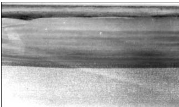
Figure 1. Crack-free longitudinal macrosection of the rail flange deposited with eight beads using an experimental flux-cored wire of the GSMF type
