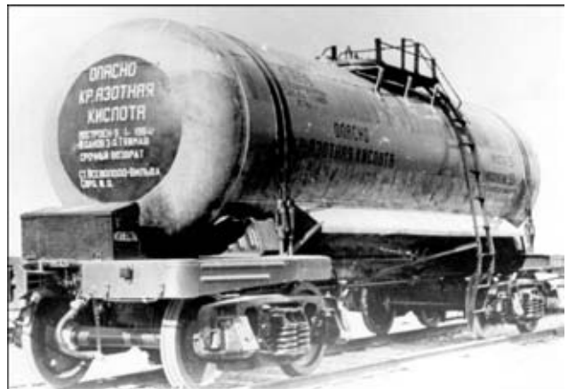
Figure 4. Tank-wagon for transportation of aggressive chemicals
