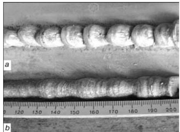
Figure 4. Disturbances (top view), arising on the surface of a weld on aluminium alloy in EBW in the downhand position at the speed of 4 \text{ mm/s} : a — by static electron beam; b — with electron beam scanning ( f_1 = 180 \text{ Hz} )
