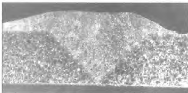
Figure 3. Macrostructure of welded joint produced by EBDM method
