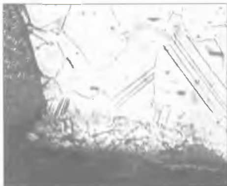
Figure 5. Character of fracture of alloy 59 after testing in a peptisation reactor at the Company «Titan» ( \times 120 )
