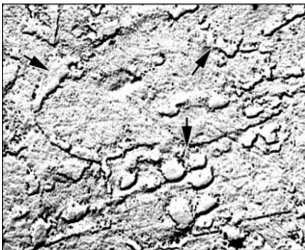
Figure 8. Metal of the incomplete refining region damaged by creep pores (carbon replica; service life 150,000 h; welding under standard conditions; base metal — steel 15Kh1M1F) ( \times 6000 )
