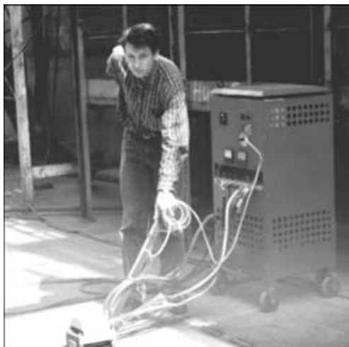
Figure 7. Induction heating HF source with a heating device
