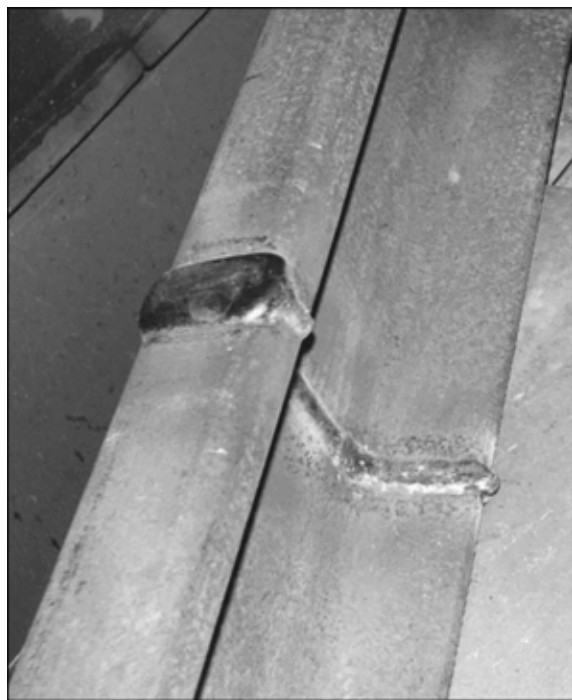
Figure 2. Butt joint in rail of the R-65 steel made by electric arc welding using embedded electrode
