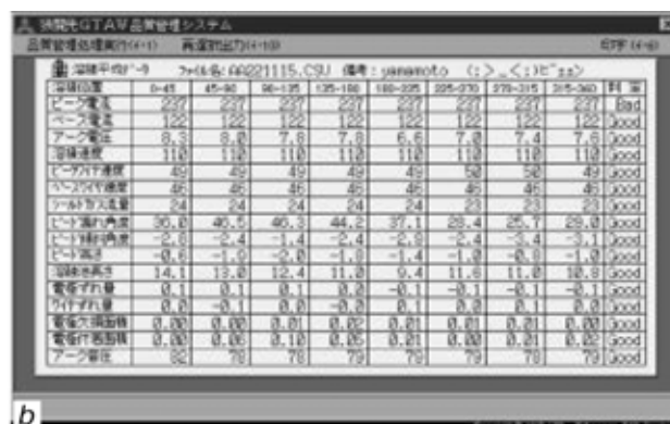
Figure 8. Display examples of welding control system: a — welding condition display; b — record of automatic welding
