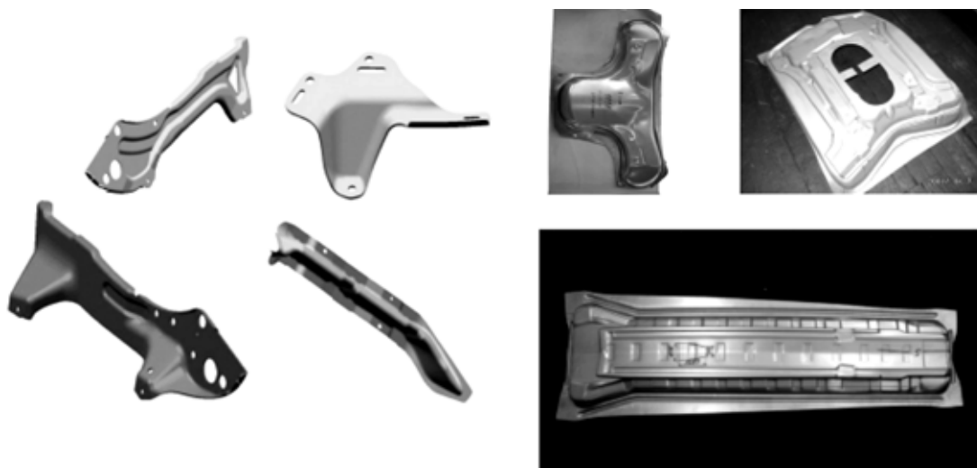
Figure 5. Laser 3D cutting application: various elements of car armchair and body of deep-drawing, Zn-coated and carbon steel 0.8 + 3 mm (3D, f = 5'' )
