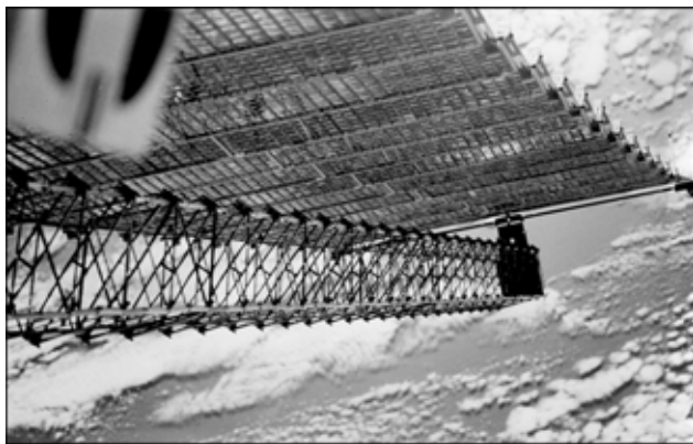
Figure 15. Hinged truss developed by PWI and shown as part of the reusable solar battery of «Mir» station
