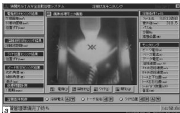
Figure 8. Display examples of welding control system: a — welding condition display; b — record of automatic welding
