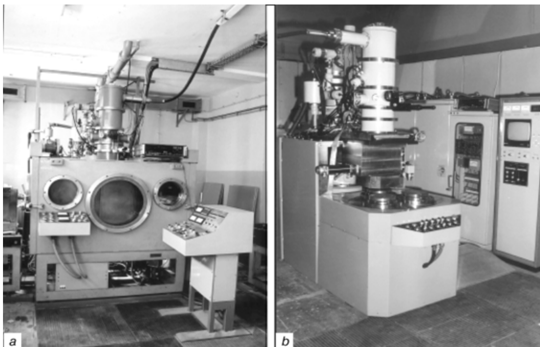
Figure 1. EBW machines designed and built at the Welding Institute in Gliwice: a — EB Welder SE60/10: chamber interior dimensions of 1500×1000×1000 mm, with X, Y axis work envelope (650×500 mm), rotary axis (A and C rotary table with jaw chuck), triode type gun (direct heating, 10 kW/60 kV), optics, beam oscillation generator, pumping system (mechanical pump + Root's + diffusion pump, automatic control) and work cycle of 10 min × 5·10 -3 hPa, vacuum in chamber of 2·10 -3 hPa and gun space vacuum of 2·10 -5 hPa; b — EB Welder SE60/15: system with three-position rotary table and programming of welding parameters, triode type gun (direct heating, 15 kW/60 kV), optics, work envelope (Y axis moving gun of 110 mm, h = 50 mm, ring Ø = 220 mm max and h = 300 mm, shaft Ø = 40 mm max), pumping system (mechanical pump + Root's + diffusion pump, automatic control), work cycle of 15 s × 2·10 -3 hPa, vacuum in chamber of 2·10 -3 hPa and gun space vacuum of 2·10 -5 hPa
