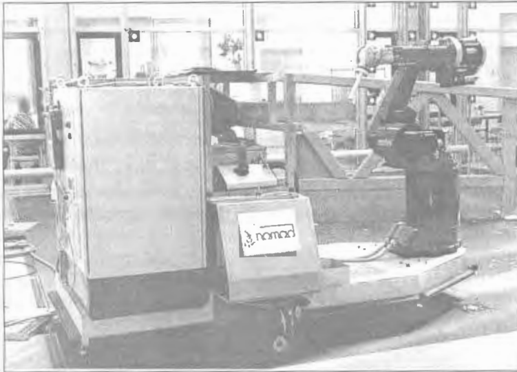
Figure 1. Robocar carrying the robot, welding equipment and control systems
