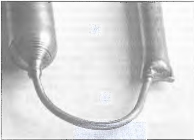
Figure 4. Brazed joint between a capillary 2 mm in diameter and tubes 5.4 and 10 mm in diameter
