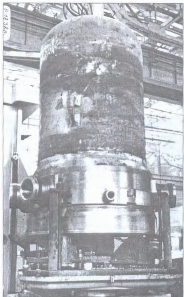
Figure 4. Stamped-welded body of transport nuclear power reactor of bimetal rolled metal 18Kh2MA + 00Kh18N10T in stand after final mechanical treatment
