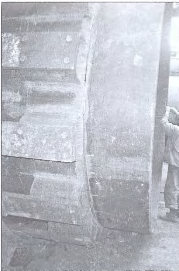
Figure 6. Fragment of a kiln with grooving for making a circumferential weld
