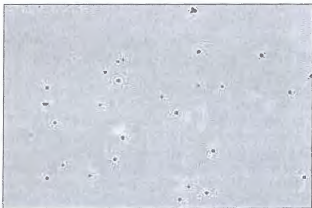
Figure 3. Non-metallic inclusions in the zone of 33KhSN2MA welded joint with weld metal of 10KhGNMAFCh type ( \times 1500 )
