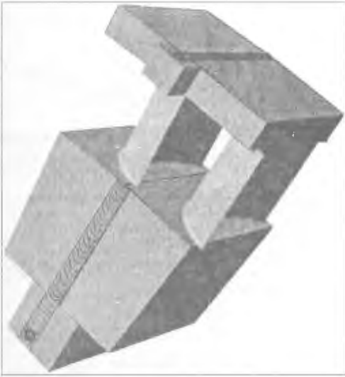
Figure 1. Model of a pack of two blades (run-on and run-off tabs are located at butt joints)
