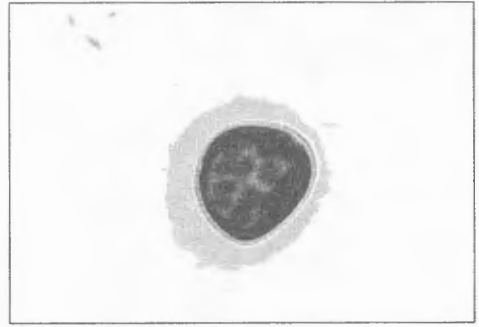
Figure 3. Illustration of region around NMI of composition different from that of matrix ( \times 3000 )
