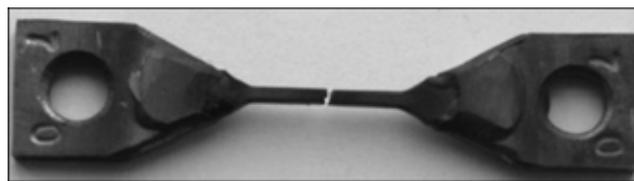
Figure 3. Appearance of ChS-70 specimen after high-temperature tests
