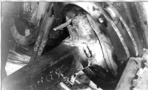
Welded-up crack in the automatic coupler case in the tail piece transition to the head
