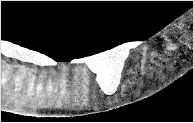
Figure 1. Macro-section of neck fragment of energy absorber body with renovated areas of internal surface
