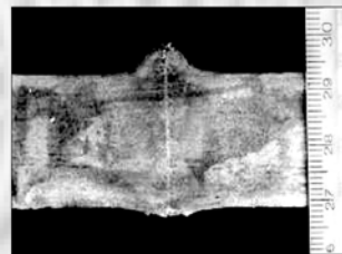
Macrosection of a welded joint made under water
