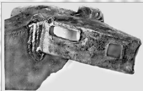
Welded-up through-thickness crack in the rear part of automatic coupler head
