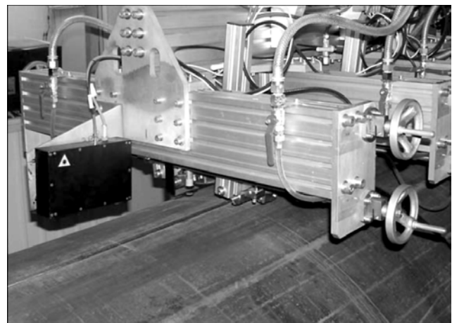
Figure 3. TV sensor on the first acoustic module of NK 360 unit
