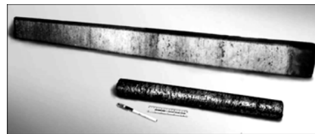
Appearance of 140 × 160 mm slab and 70 mm diameter cylindrical ingot of EBCHR high-speed steel R6M5
