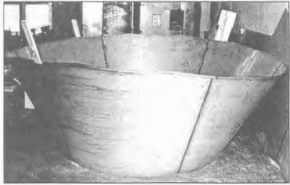
Figure 13. General view of the welded conical shell before corrugation formation
