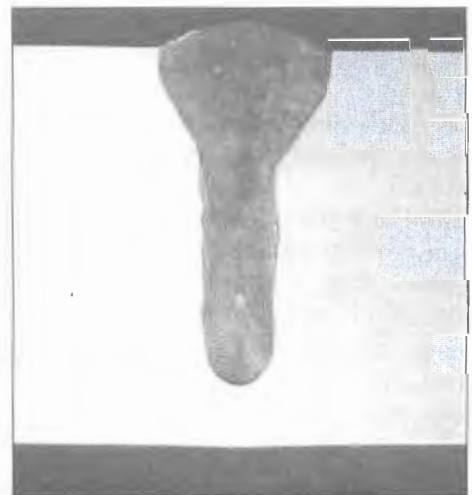
Figure 4. Bead-on-plate weld on AA6082 ( t = 12 mm, P_L = 10 kW, v_w = 3 m/min)
