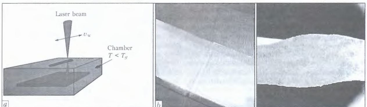
Figure 5. Schematic representation of butt joining process of plane glass (a) and its view under raster electron microscope (b)
