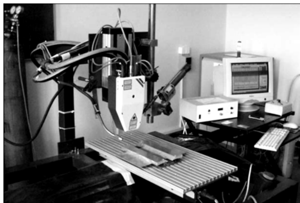
Figure 2. View of experimental setup for HPDL welding of the aluminum alloy butt joints
