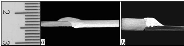
**Figure 5.** Macrosection of welded joints from dissimilar materials of stainless steel-aluminium alloy AMg6 produced by the schematic given in Figure 3: *a* — billet assembled with an overlap; *b* — billet before welding assembled using thread
