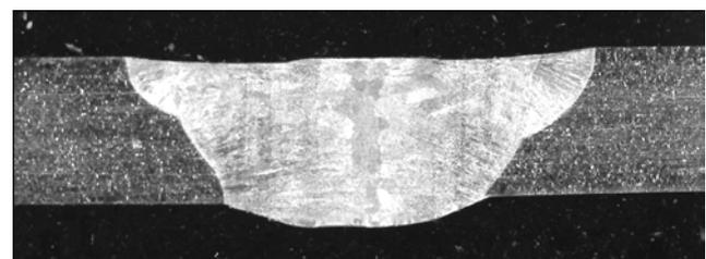
**Figure 3.** Photomicrograph of a typical weld specimen cross-sectioned at A-A showing bead profile ( $\times 10$ )
