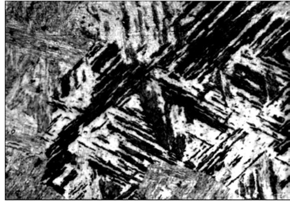
**Figure 1.** Microstructure of steel 03Kh12N8M2GST (prototype of weld metal) ( $\times 500$ )
