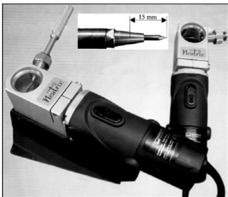
Owing to its mobility Neutrix instrument is ideal for mounting operations and other tasks which require a portable grinding machine. For stationary operation
