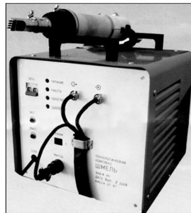
Technical characteristics of the system are as follows: working frequency of 26–28 kHz, output power of 500 W, power voltage of 220 V, weight of 21 kg, overall dimensions of 36 × 390 × 420 mm.
