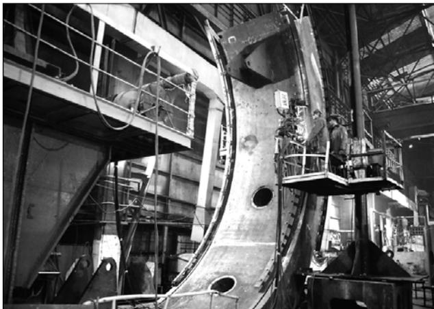
**Figure 3.** Working moment of ESW of standard workpiece under workshop conditions
