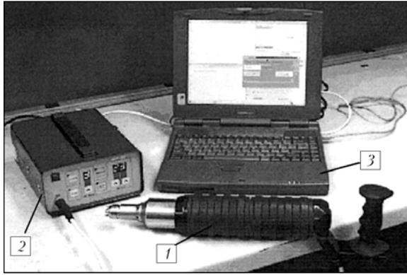
**Figure 2.** Equipment of 0.3 kW power for HFMP of welded joints of metal structures: 1 — manual tool with a piezoceramic radiator; 2 — ultrasonic generator; 3 — computer
