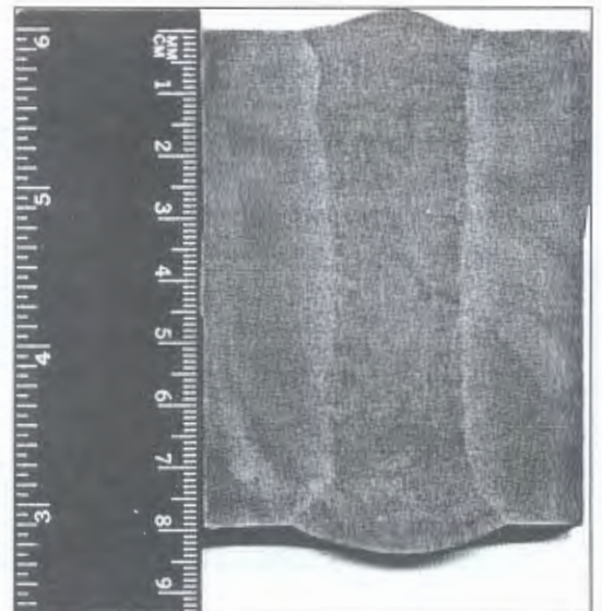
Figure 5. Macrosection of welded joint (material to be welded is steel St3 80 mm thick)
