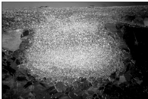
Figure 8. Metal macrostructure of deposited layer of M1 copper (x5)
