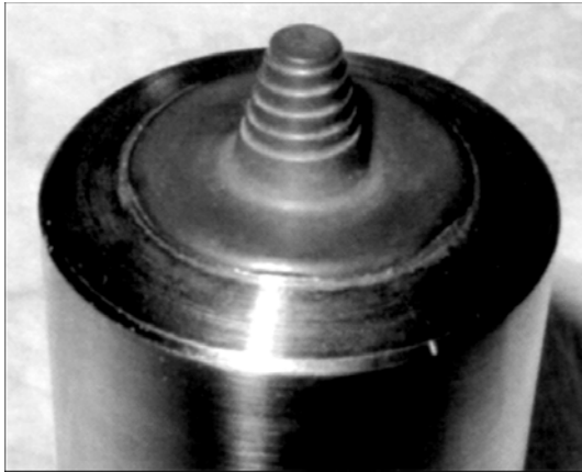
Figure 8. Appearance of the tool from polycrystalline cubic boron nitride [2]
