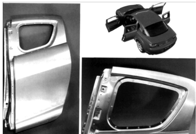
Figure 11. Joints made in Mazda RX-8 car using spot FSW [2]
