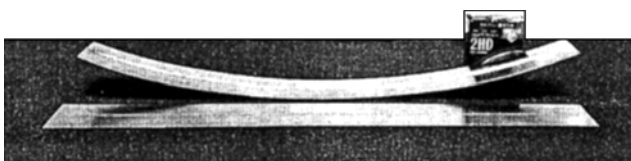
Figure 3. Comparison of angular deformation at FSW (lower sample) and MIG welding (aluminium alloy of 6000 series, 2 mm thickness)
