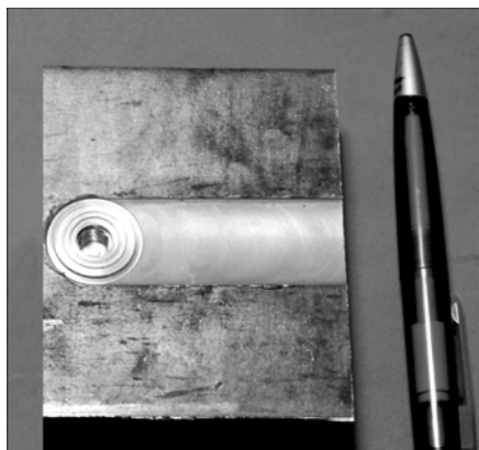
Figure 3. Exposed surface of L6 brass joint produced by FSW
