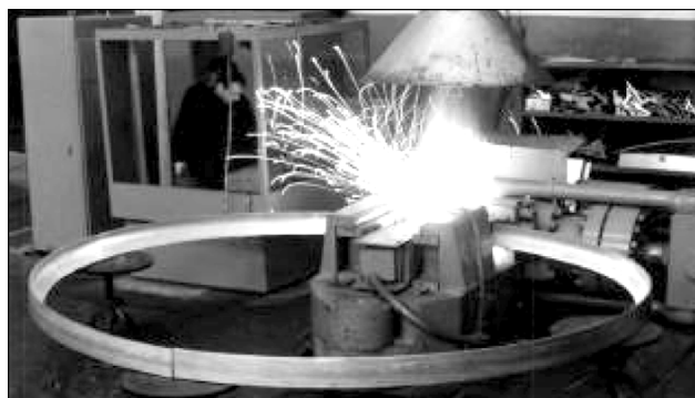
Flash butt welding of frames using machine K393
