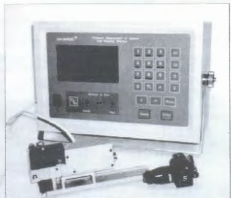
General view of ultrasonic device for monitoring of stresses
