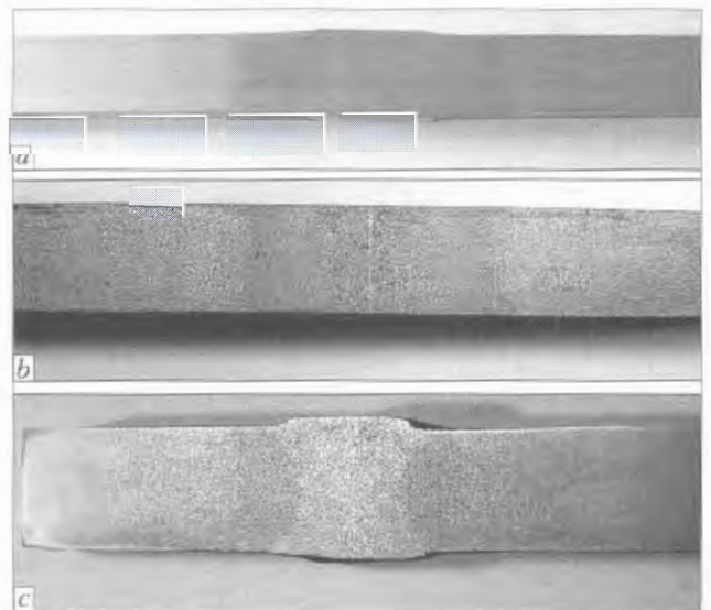
Figure 4. Macrosections of pipe welded joints (x2): a – batch #1, mode A; b – batch #2, mode A; c – batch #2, mode B
