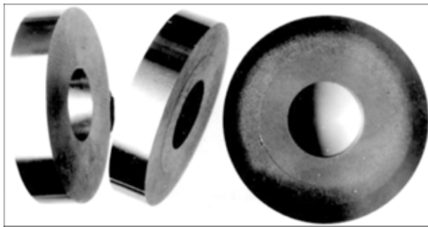
Figure 1. Roller for determining tribotechnical characteristics of friction-sliding pairs: external diameter of 50 mm, thickness of 12 mm
