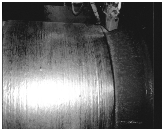
Figure 3. Appearance of deposited on water turbine shaft corrosion-resistant layer
