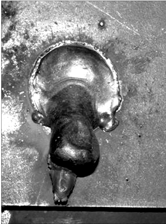
Figure 2. Spot joint made in vertical position under the conditions used for ASW in flat position
