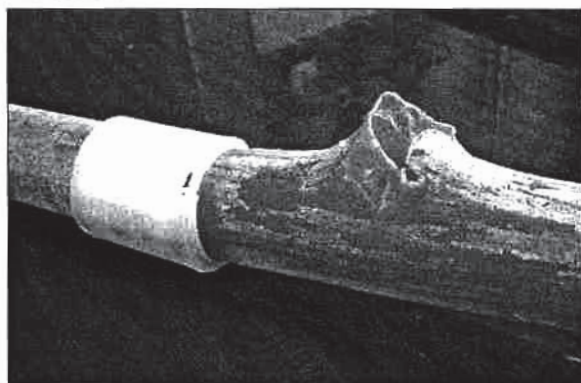
Figure 4. Sample of the joint on PE-Xa grade structured polyethylene pipe with outer diameter of 50 mm and wall thickness of 4.6 mm after hydraulic tests
