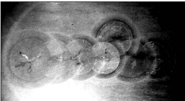
Figure 1. Transverse macrosection of specimen of steel 35L of 500 × 300 × 500 mm size with hot cracks formed after ESW of holes of 50 mm diameter and 500 mm depth
