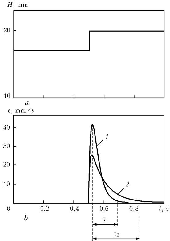
**Figure 2.** Stepwise change in distance  $H$  between the nozzle and weld pool (a), and response of deviation  $\varepsilon(t)$  to this change (b): 1 –  $S_s = -0.015$ ; 2 –  $-0.045 \text{ V/A}$
