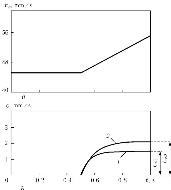
Figure 1. Linear change in electrode feed speed  $v_e$  (a), and response of deviation  $\varepsilon(t)$  to this change (b): 1 -  $S_s = -0.025$ ; 2 -  $-0.045$  V/A
