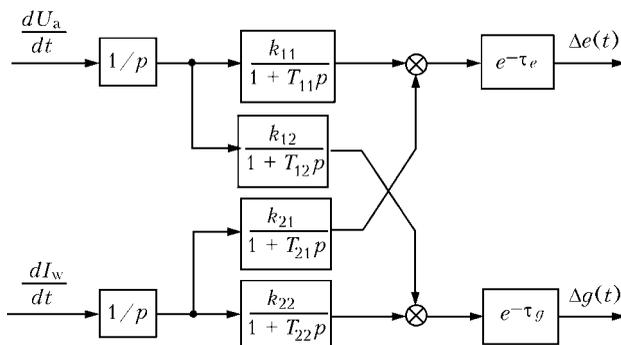
Figure 2. Structure chart of the dynamic weld reinforcement formation model
