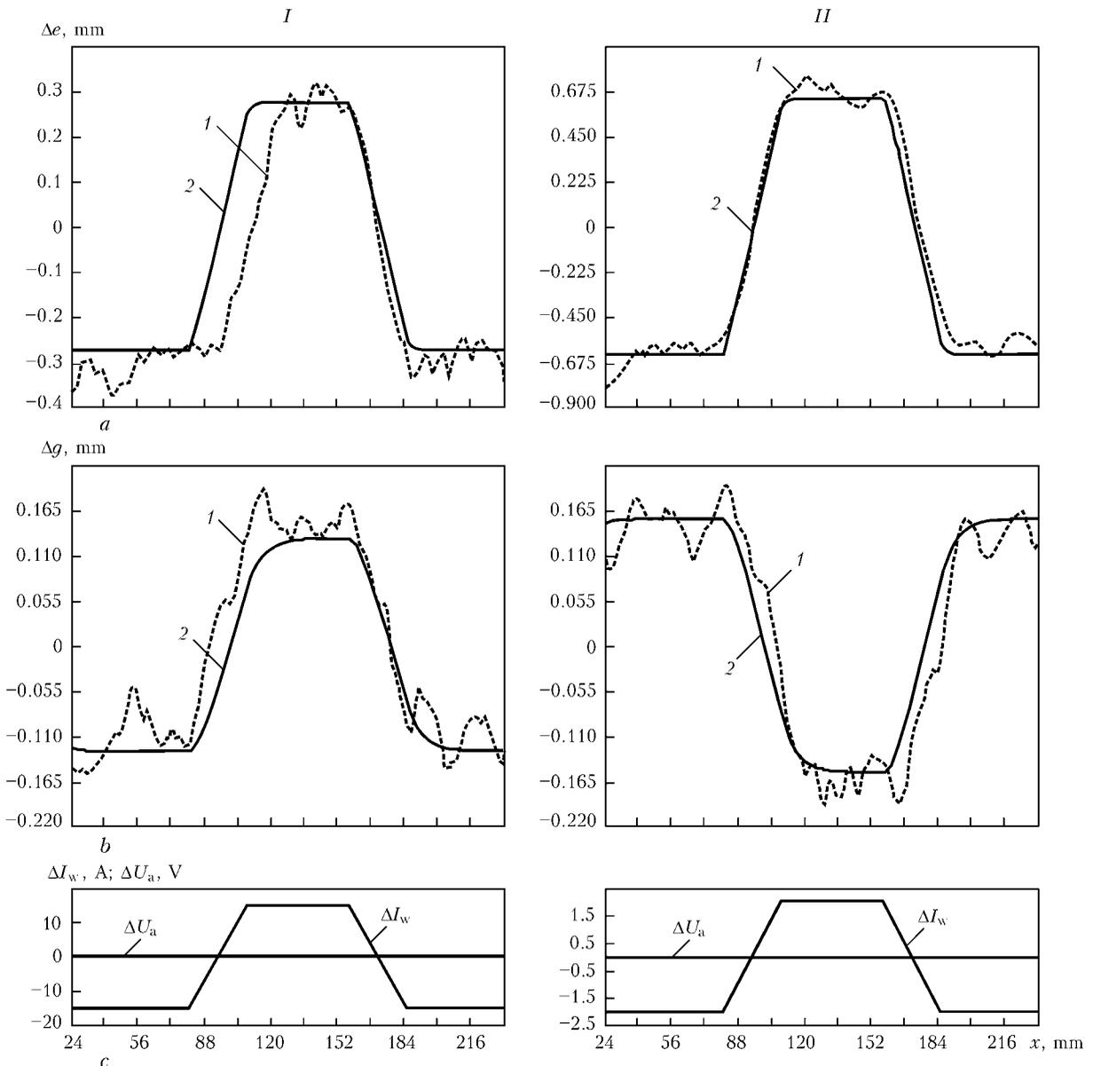
**Figure 1.** Results of identification of parameters of dynamic links of the weld reinforcement formation model for a pulse of welding current (I) and voltage (II); a, b – variations in width and height of the reinforcement bead, respectively; c – increments of welding current and voltage adjustment actions, respectively: 1 – reaction of dynamic links of the model; 2 – geometric parameters of the reinforcement bead measured with LTS
