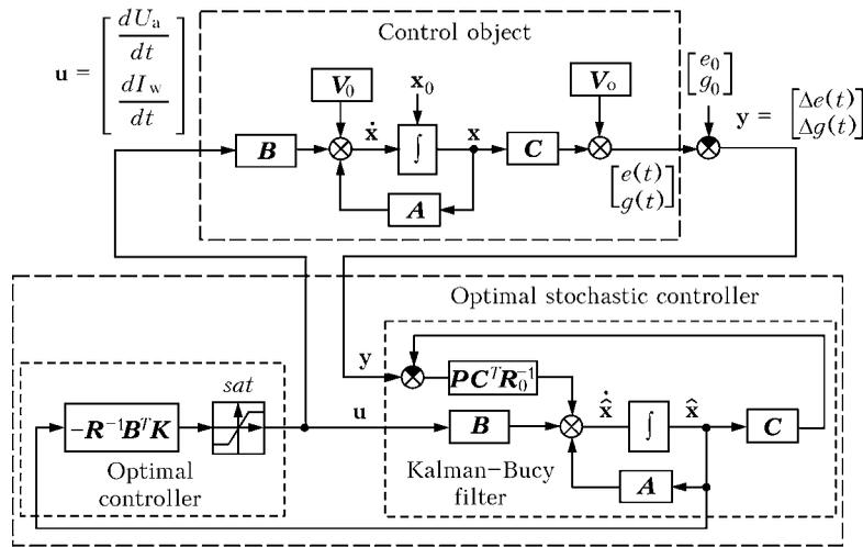
Figure 3. Structure chart of the optimal ACS model
