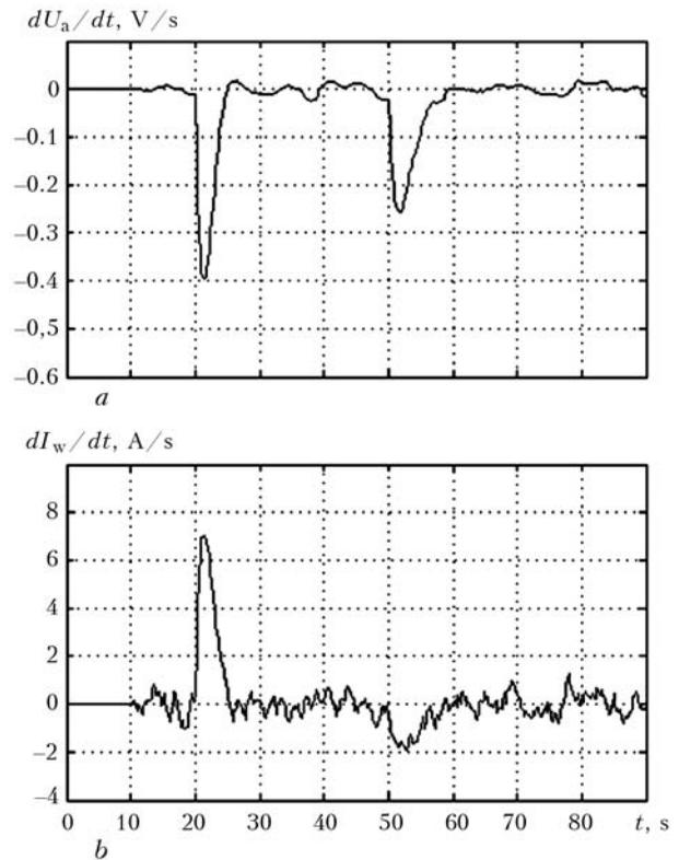
**Figure 6.** Curves of voltage (a) and welding current (b) signals in optimal ACS
