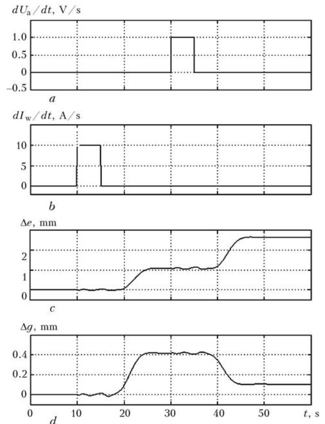
Figure 4. Transient characteristics of the dynamic control object model: a, b – voltage and welding current control actions, respectively; c, d – variations in weld width and height, respectively
