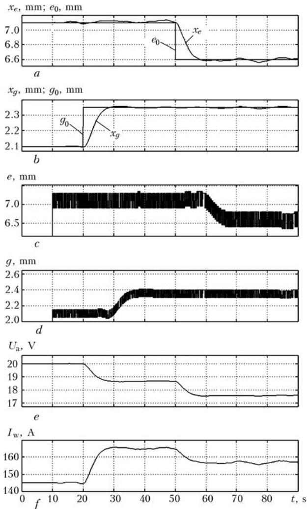
**Figure 5.** Curves of the transient process in optimal ACS with a change in master controls  $e_0$  and  $g_0$  at the 20th and 50th second:  $a, b$  – width  $x_e$  and height  $x_g$  of the bead at a current time point;  $c, d$  – signals of observation of width and height of the bead;  $e, f$  – adjustment actions
