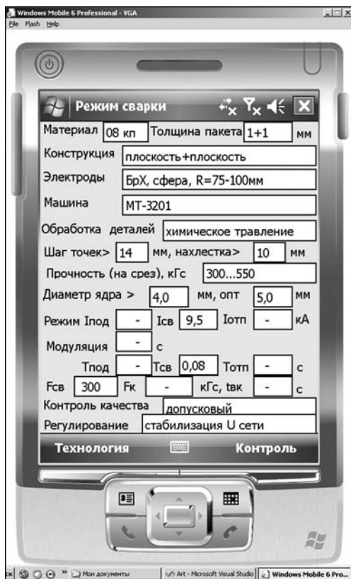
Figure 4. Data on welding technology on pocket PC display
