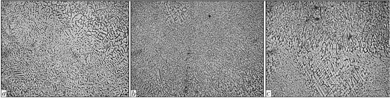
**Figure 3.** Microstructure ( $\times 320$ ) of weld metal of 12Kh18N12T steel tubular joint produced by orbital TIG welding for four passes: *a*, *b* – weld metal, respectively, after the first and second passes; *c* – at the boundary of the third and fourth passes
