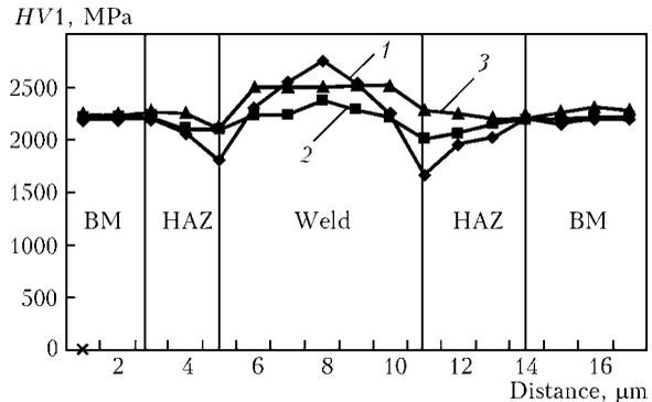
**Figure 5.** Distribution of microhardness of 12Kh18N12T steel tubular joints (specimen 47) made by orbital TIG welding for one (1), two (2) and three (3) passes
