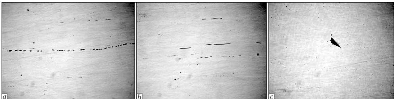
**Figure 2.** Microstructures ( $\times 500$ ) of base and weld metal with nonmetallic inclusions in them: *a* – chains of oxides in BM along the rolling; *b* – sulphides in BM elongated along the rolling; *c* – inclusions of corundum and silicates in a single-pass metal
