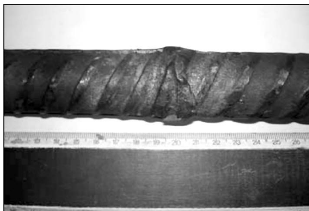
Figure 3. Appearance of welded joint of reinforcement of 32 mm diameter of steel 25G2S
