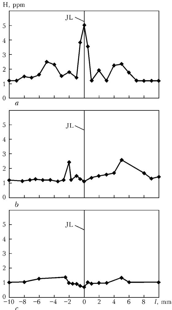
Hydrogen distribution in the zone of FBW joints on steel 10G2FB at upsetting of 0.18 (a), 0.38 (b) and 1.28 (c)
