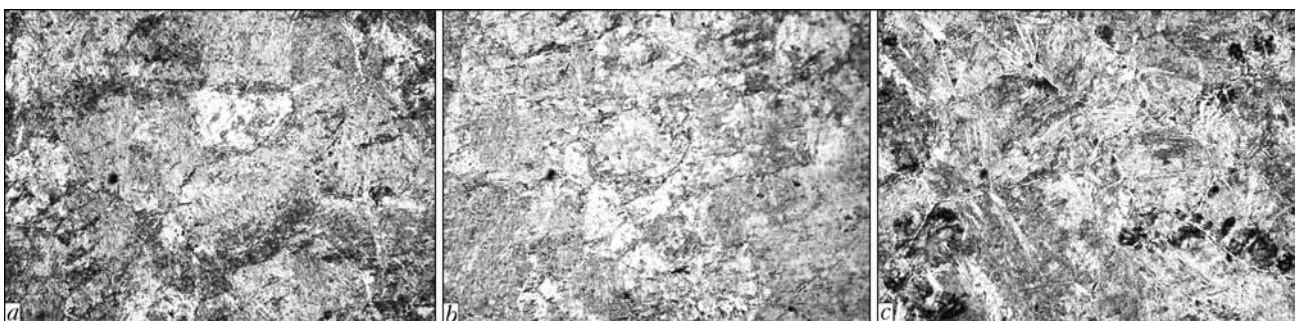
Figure 2. Microstructures ( \times 500 ) of HAZ metal of wheel steel of type T at w_{6/5} = 20.0 (a), 11.1 (b) and 7.7 (c) °C/s
