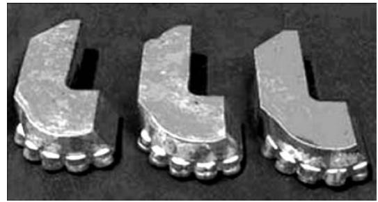
Figure 5. Blades of drill bits with DHAC brazed into them
