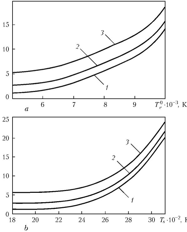
Figure 5. Heat flow on steel anode surface versus electron temperature  $T_e^0$  in the near-anode plasma layer (a) and anode surface temperature  $T_s$  (b) in argon welding: 1-3 – same as in Figure 3
