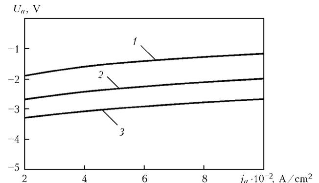
**Figure 4.** Anode potential drop  $U_a$  versus anode current density  $j_a$  for steel anode in argon welding ( $T_s = 2472$  K): 1 –  $T_e^0 = 6 \cdot 10^3$ ; 2 –  $7 \cdot 10^3$ ; 3 –  $8 \cdot 10^3$  K
