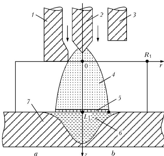
**Figure 1.** Schematics of plasma (a) and TIG (b) welding: 1 – plasma-shaping nozzle; 2 – refractory electrode (cathode); 3 – shielding gas nozzle; 4 – arc column; 5 – anode region of the arc; 6 – weld pool; 7 – workpiece (anode)
