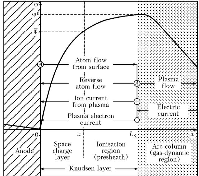
**Figure 2.** Structure of plasma presheath, particle flows and distribution of potential in the anode region of the welding arc:  $\bar{\varphi}$  – value of potential at the space charge boundary layer; A – atoms; + – ions; – – electrons; the rest of the designations are given in the text
