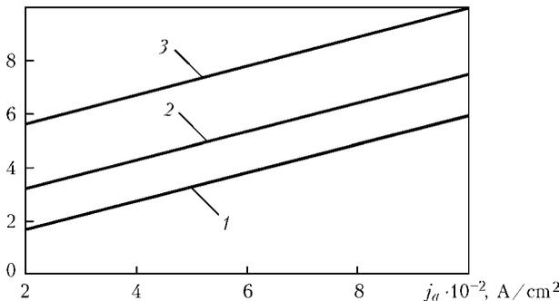
Figure 6. Heat flow to the steel anode surface versus current density  $j_a$  in it in argon welding,  $T_s = 2472 \text{ K}$ : 1-3 – see Figure 3
