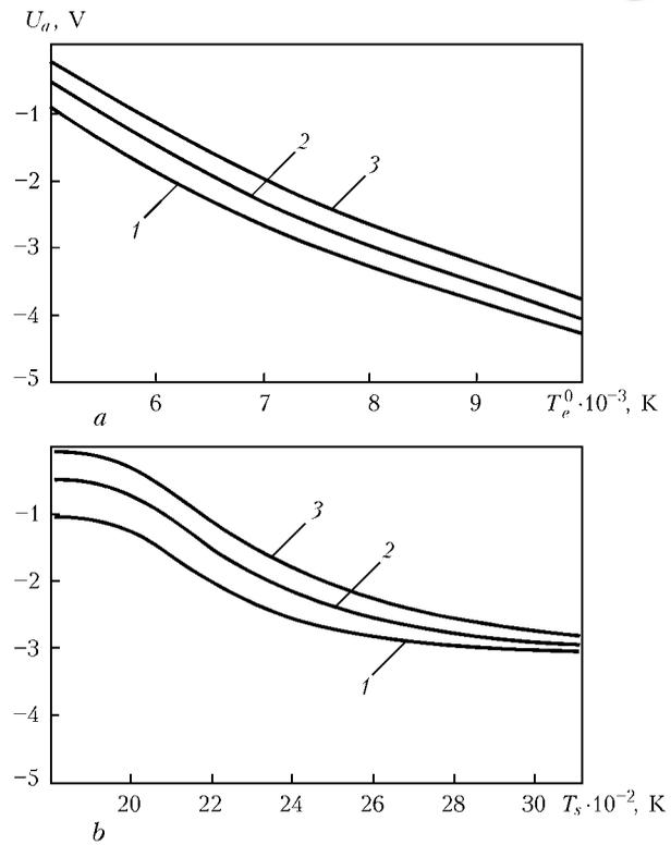
**Figure 3.** Anode potential drop  $U_a$  versus electron temperature in the near-anode plasma layer (a) and temperature of its surface (b) for steel anode in argon welding: a – 1 –  $j_a = 200$ ; 2 – 500; 3 – 1000 A/cm<sup>2</sup> at  $T_s = 2472$  K; b – 1–3 – see Figure 3, a, but at  $T_e^0 = 7 \cdot 10^3$  K
