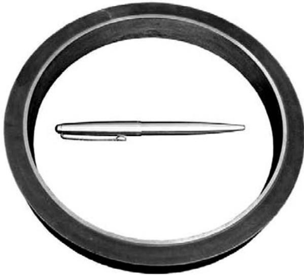
Figure 12. Transverse macrosection of bushing
