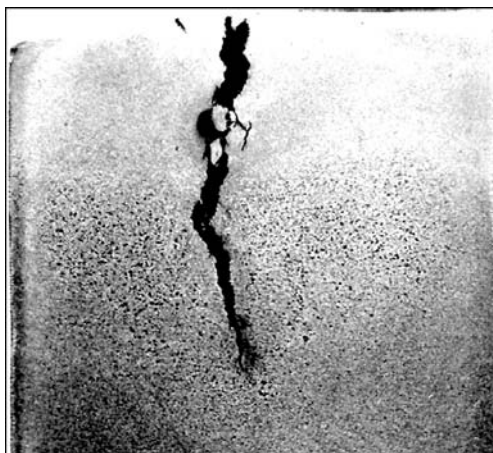
Figure 1. Macrosection ( \times 1.5 ) of the welded joint on steel 12Kh1MF with creep crack in the weld metal (live steam pipeline, 190,000 h running)
