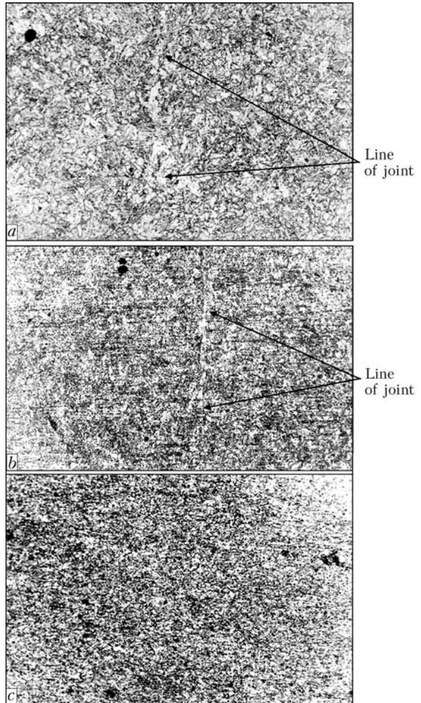
Figure 6. Microstructures ( $\times 150$ ) of welded joint near external edge (a), in central area (b) and parent metal (c)
