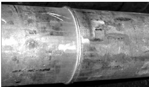
Figure 1. Welded joint of steel X70 pipes of  $\varnothing 168 \times 7$  mm
