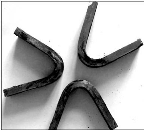
Figure 3. Results of bend tests of welded joint
