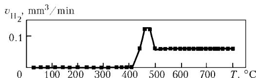
**Figure 3.** Spectrum of thermal desorption of residual hydrogen from deposited metal of one-layer weld made with electrode IP 16
