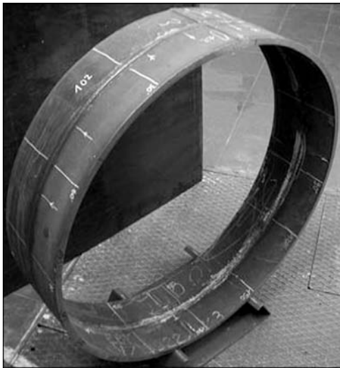
Figure 6. Sample made by semi-orbital hybrid welding
